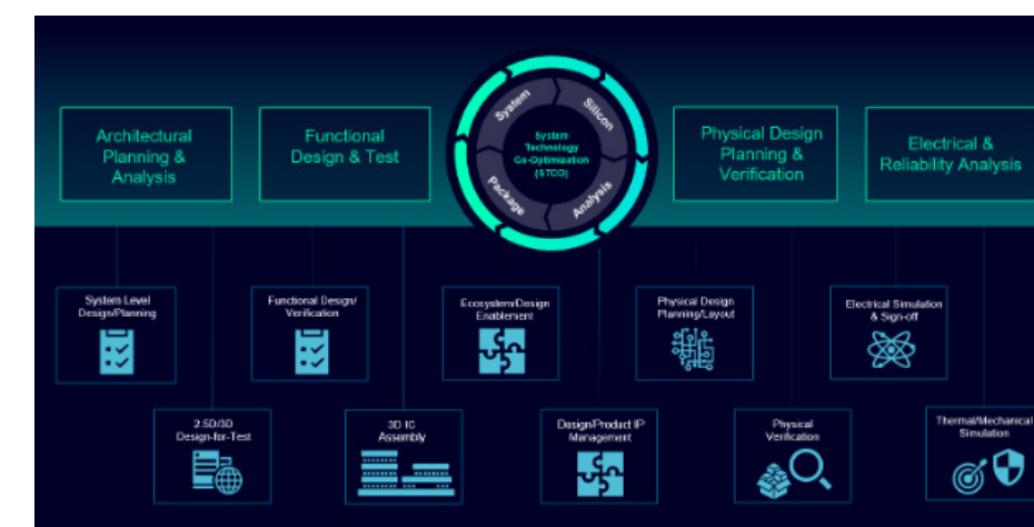
Figure 1: 3D IC heterogeneous integration requires a co-design and co-optimization approach (STCO).
