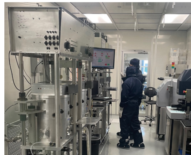
Figure 2: This Class 1000 etch bay is outfitted with customized equipment, such as this dual chamber, silene based oxide deposition system.
