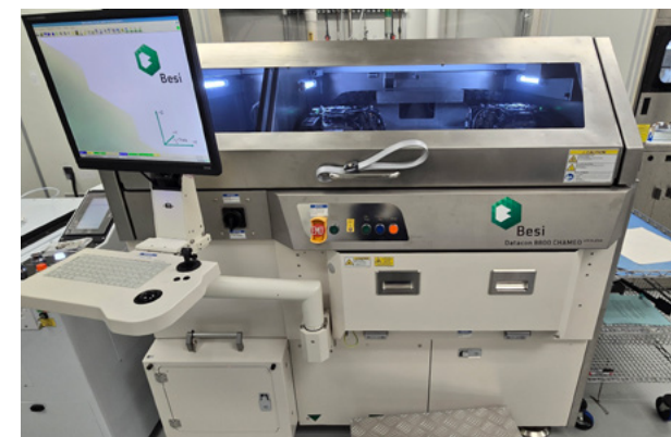
Figure 4: The Besi Datacon 8800 CHAMEO ultra plus is an advanced room-temperature hybrid bonding system that addresses increased demands for performance, speed, accuracy, and warpage control in fine-pitch copper interconnects with submicron pad sizes.
